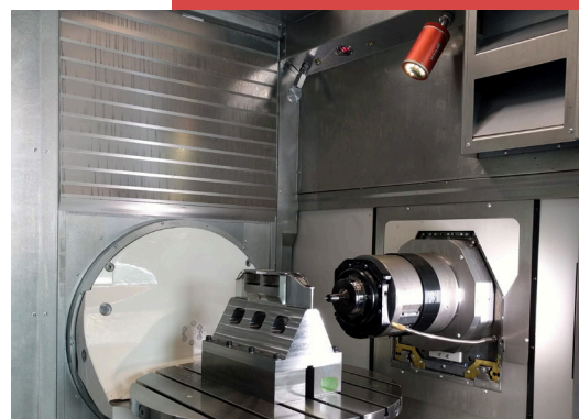
Installation of RWC 2.0 in 5-axis milling machine
